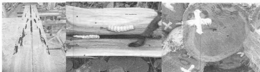
Figure 7 : The infestation of teak wood by Teak Beehole Borer (TBB)
