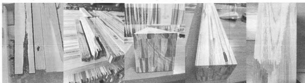
Figure 9 : Glulam (glued laminated timber) from small and insect-damaged teak logs
